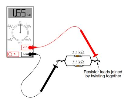
Follow-up question: how much resistance would you expect the ohmmeter to register if there were *three* similarly-sized resistors connected in parallel instead of two? What if there were *four* resistors?
