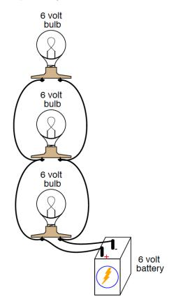
Calculate the total amount of current that the battery must supply to this parallel circuit:
