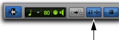
Link Timeline and Edit Selection enabled in the Score Editor window
