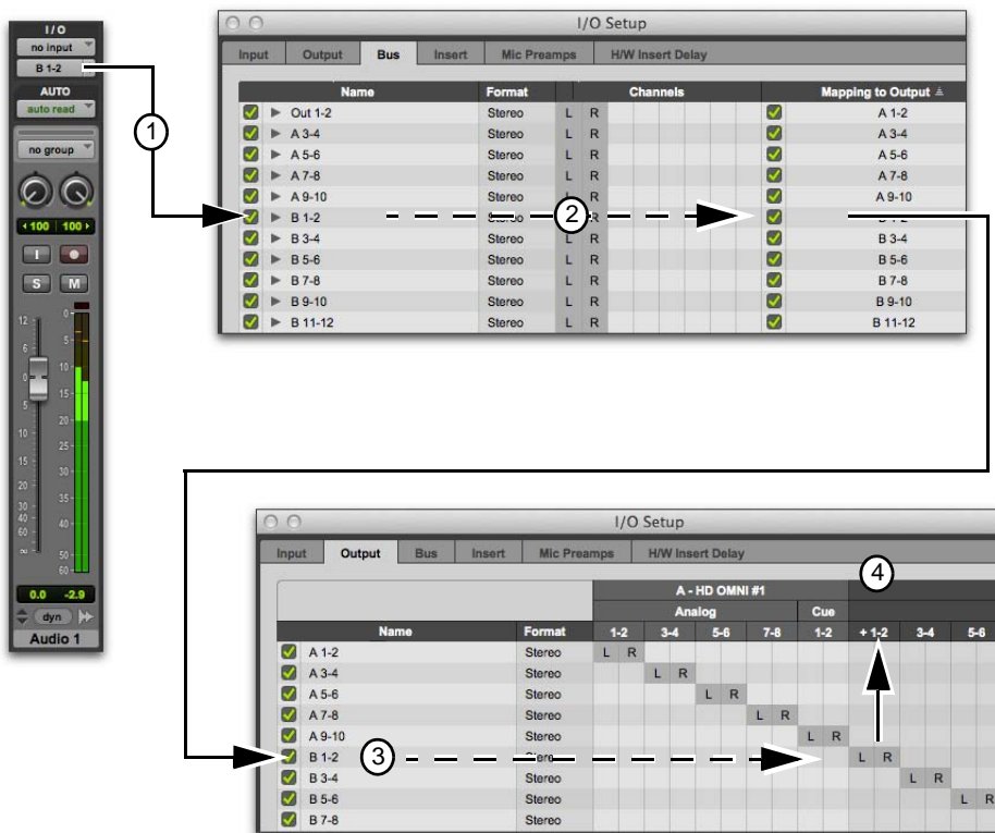
Output signal path from an audio track to a physical output as mapped in I/O Setup
