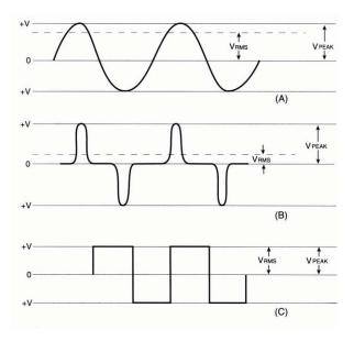
Look at the string of narrow pulses (Waveform B) in the figure. The voltage spends much more time at zero than at some positive or negative voltage. Even though the peak voltage of this pulse waveform is the same as the sine wave above, the RMS value of the pulse waveform is lower. It will indicate lower on a VU meter, and it sounds quieter than a sine wave with the same peak amplitude. This is why a drum may be at the correct volume in a mix but appear to read low on the VU meter.
