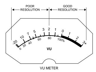
This is excellent resolution when reading steady tones, but not very useful when working with a recording medium that's capable of handling a dynamic range of better than 90 dB. There's virtually no usable resolution below -10 VU, so if we take it on faith that we have at least 10 dB of headroom above 0 VU even though we can't see it on the meter, we have an indication of only about a 13 dB headroom range.
